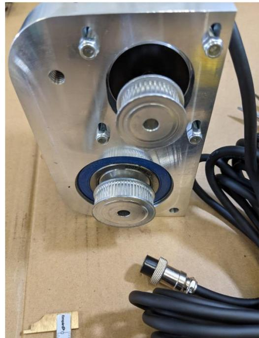
Place the belt on the gears smooth side out.
