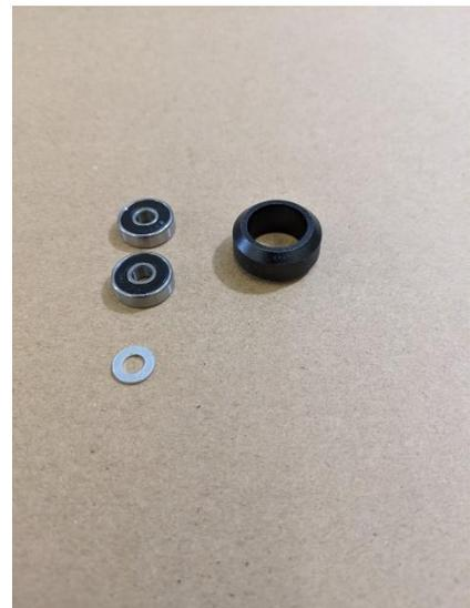
Locate the tail stock slider plate. Place a v wheel on a M5x25 machine screw, followed by a standard spacer. Screw it into the threaded hole on the corner of the tail stock slider plate. Repeat the process with a second v wheel.
