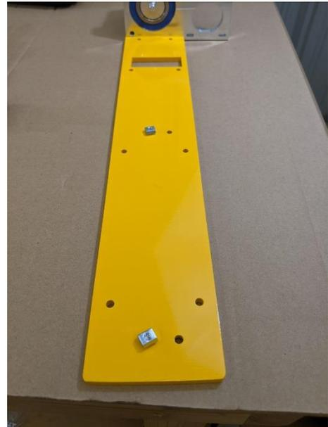
Line up the nuts with the slot on the extrusion and slide it onto the base plate. Tighten the screws.
