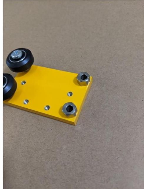
Take an eccentric spacer and insert it into the larger hole opposite of the v wheels you installed earlier. Make sure the notch on the eccentric spacer is facing away from the installed v wheels. Place a v wheel on a M5x30 machine screw. Place the screw through the eccentric spacer and secure with a M5 nylock. Repeat the process with the last v wheel.
