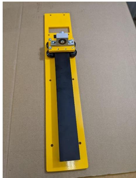
Turn the chuck assembly on its side to allow access to the mounting holes. Line up the holes at the end of the base plate with the holes on the underside of the chuck assembly. Use 2 M5x10 socket flat caps to attach the chuck assembly to the base plate.
